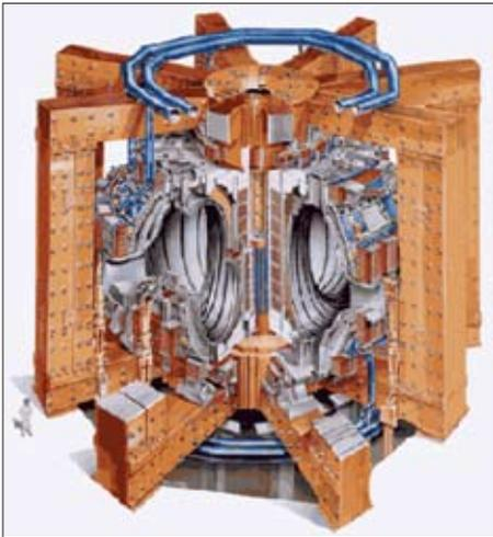
**3: A schematic diagram of the world's largest tokamak, JET, the Joint European Torus at Harwell. Large magnetic coils around the vacuum vessel generate confining magnetic fields within and around the hot plasma. (EFDA-JET)**
